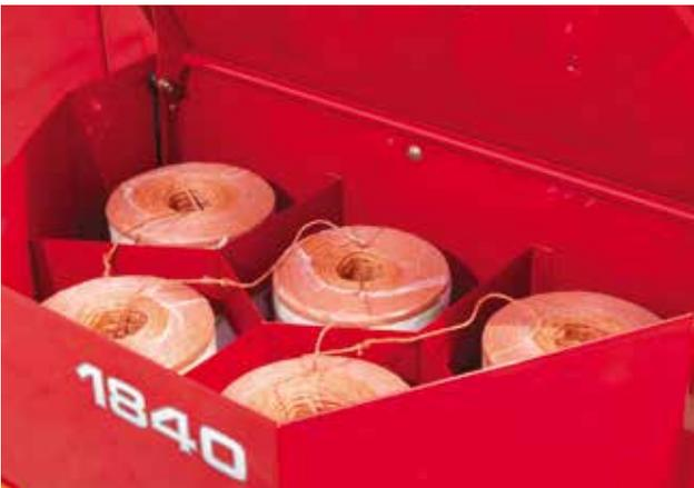
The MF1840 carries 10 balls of twine which is enough for the longest days work. The large dimension of each compartment allow 'super large' size twine spools to be used, enabling even more twine to be carried and therefore more bales produced per twine fill-up.
