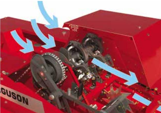
Air is drawn in from the front, flows across the knotters and out of the rear of the knotter cover.
