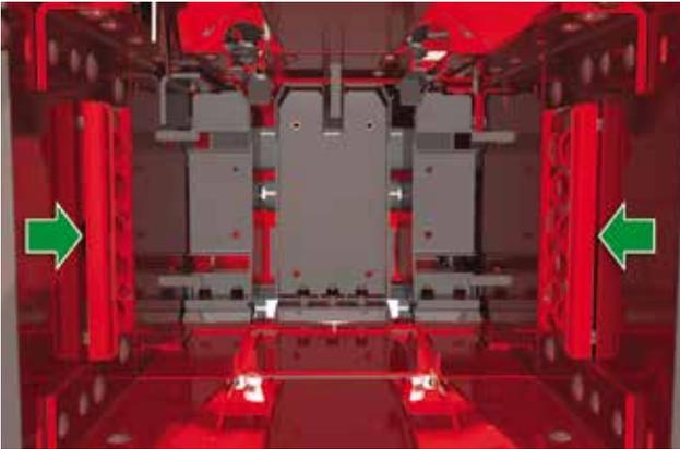
To ensure superb bale shape in all conditions and maintain consistent density, the OptiForm bale chamber is 460 mm or 30% longer when compared to the previous MF1839 baler.
