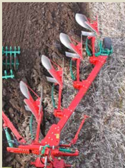
One-piece mainframe for strength and flexibility.
