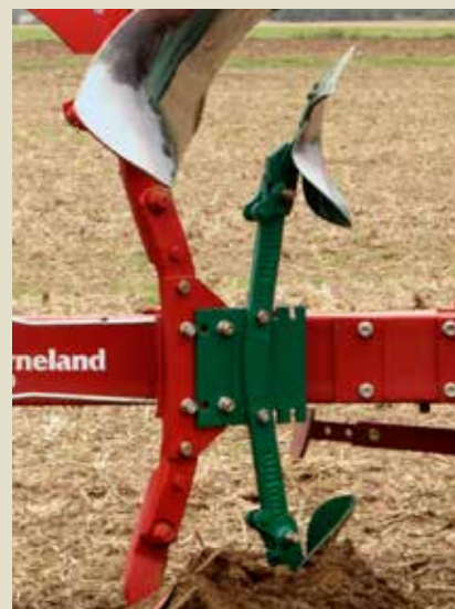
Kverneland LM is equipped with shearbolt protection.
