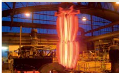
12 hours carburising heat treatment for each mouldboard.
