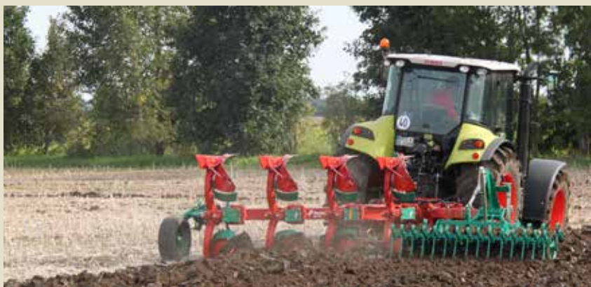
When fitted with the Packomat the EM/LM will plough and pack a seedbed all in one operation.
