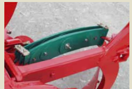
Double spring package - with 14 leaves (1400 kp)
