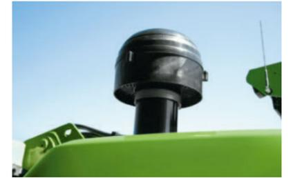
• Cyclone pre-separator for the air filter
