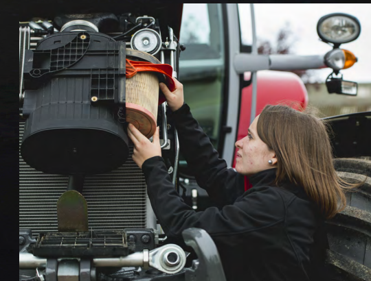
Engine air filter is easy to access and clean.
