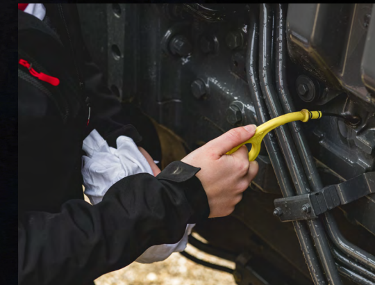
Front axle and slim waist bonnet design make oil dipstick and filter access easy.
