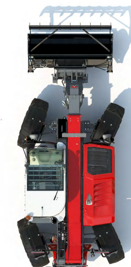
FOUR-WHEEL steering mode – for minimum turning circles.
